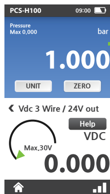
Pressure/Electrical Measurement Screen
